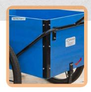
Sakaramenta has developed the Black Bull Push Cart. This heavy duty cart can carry up to 200kg. It has a big box, strengthened wheels with reinforced spokes and hubs. The tyre and the tube are the same size as the widely available mountain bike tyres. So the spare parts are locally available.
